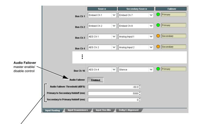
Failover controls set the conditions that comprise a loss of audio event, and also a transition back to primary channels.
