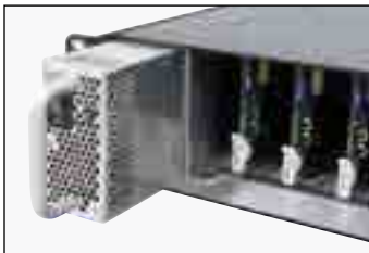
Hot-swappable power supply (with optional redundant supply) is easily replaced from front of frame
