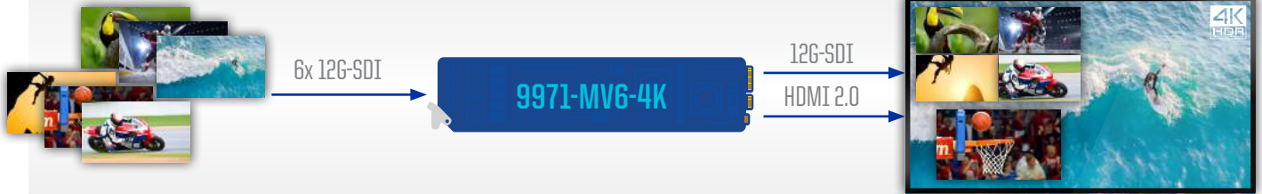
Six 12G-SDI 4K Inputs to a Single 3840x2160 UHD Display via 12G-SDI & HDMI 2.0
