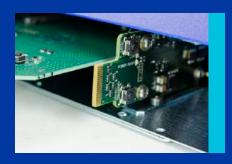
A built in network card, along with an LCD screen and front control panel that includes a rotary knob, makes navigation, status monitoring and network connectivity simple and easy to use.
