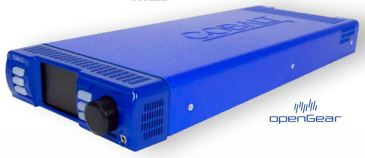
The BBG-1300-FR 1RU Enclosure Holds up to Two openGear® Cards with Standard Size Rear IO Modules, a Built In Network Card and 60 W of Available Power.
