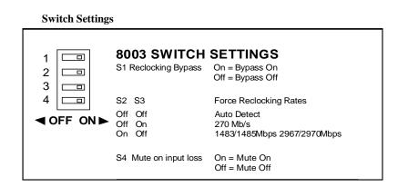
S1 – Bypasses the reclocker. ON for Bypass. OFF for reclocking.
