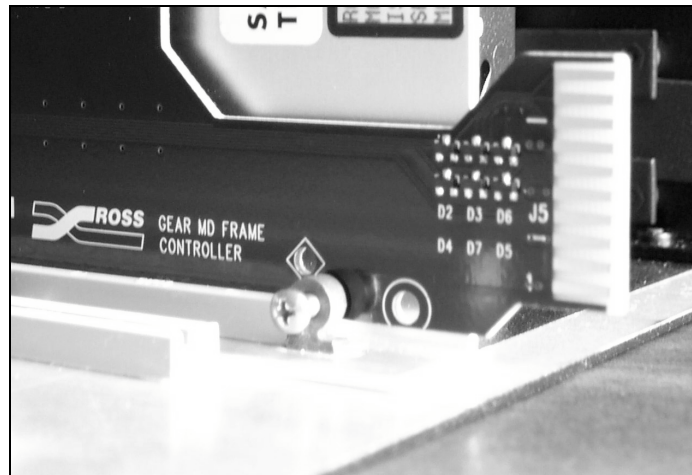
Figure 11. MFC-8320 Fan Controller Card and Unscrewed Retaining Screw
