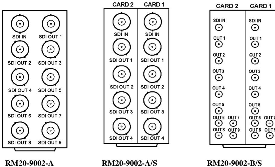
**Note:** Early versions of 9002 have some outputs as inverting. These outputs are not compatible with ASI video. Please contact product support and have card serial number on hand for more information.
