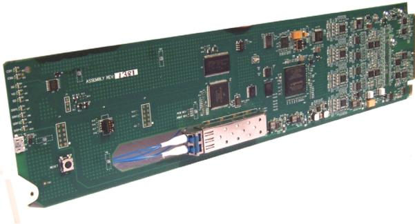
The Cobalt® 9410DA-2OE 3G/HD/SD-SDI / ASI / MADI Fiber Dual OE Transport/Distribution Amplifier with Full-Flexibility Crosspoint provides a card-based solution for high-density conversion from fiber to coax (with two independent OE channels), as well as coaxial distribution. The 9410DA-2OE is multi-rate, and supports SDI and ASI/DVB on all inputs and outputs with non-inverting outputs.
