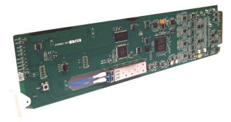
The Cobalt® 9410DA-EO 3G/HD/SD-SDI / ASI / MADI Fiber EO Transport/Distribution Amplifier with Full-Flexibility Crosspoint provides a card-based solution for high-density conversion from coax to fiber, as well as coaxial distribution. The 9410DA-EO is multi-rate, and supports SDI and ASI/DVB on all inputs and outputs with non-inverting outputs.
