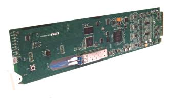
The Cobalt® 9410DA-0E 3G/HD/SD-SDI / ASI / MADI Fiber OE Transport/Distribution Amplifier with Full-Flexibility Crosspoint provides a card-based solution for high-density conversion from fiber to coax, as well as coaxial distribution. The 9410DA-OE is multi-rate, and supports SDI and ASI/DVB on all inputs and outputs with non-inverting outputs.
