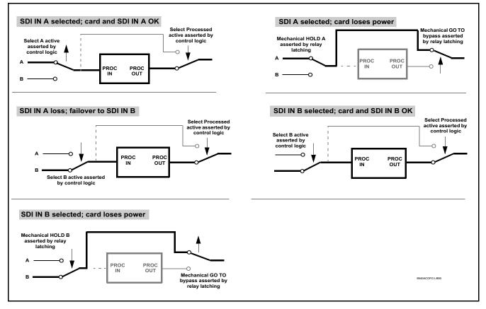
Figure 1-2 Auto-Changeover Function and Signal Flow
