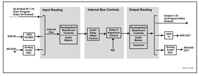
Figure 1-6 Basic Audio Processing Block Diagram
