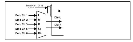
Figure 1-7 Audio Down Mix Functional Block Diagram with Example Sources
