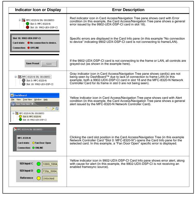
Figure 3-8 DashBoard<sup>™</sup> Status Indicator Icons and Displays
