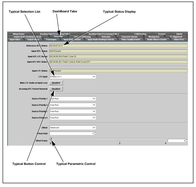
Figure 3-2 Typical DashBoard Tabs and Controls
