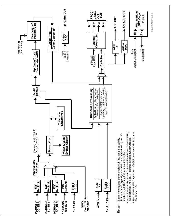
Figure 1-1 9902-UDX-DSP-CI Functional Block Diagram
