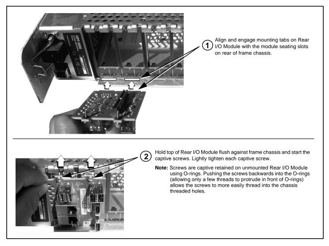
Figure 2-1 Rear I/O Module Installation
