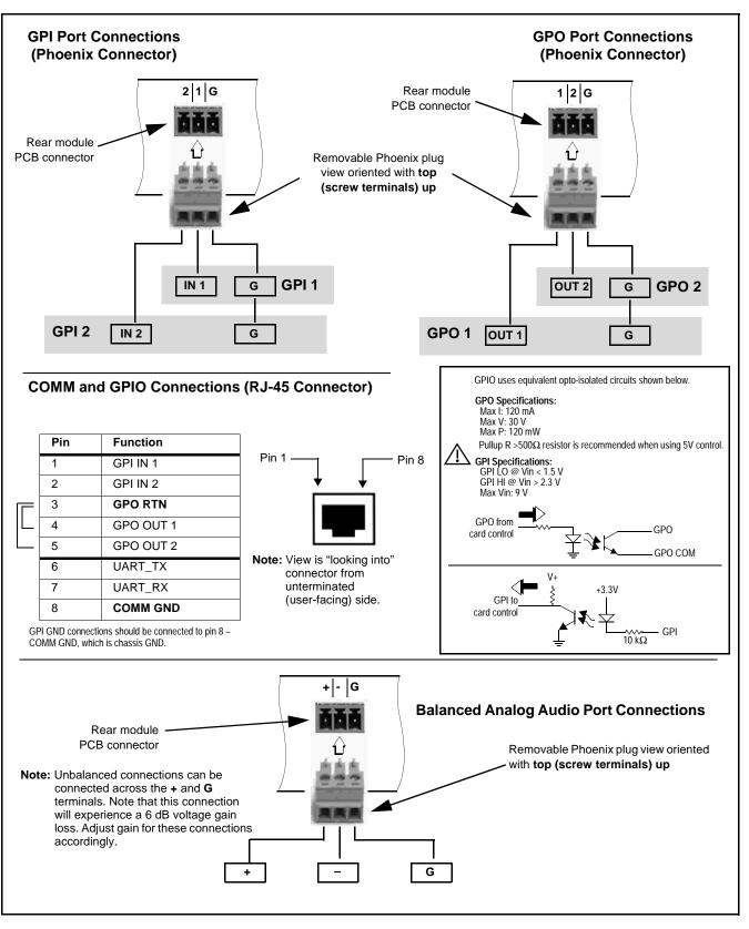
Figure 2-2 COMM, GPIO, and Analog Audio Connector Pinouts
