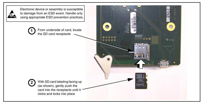
Figure 3-10 SD Card Installation
