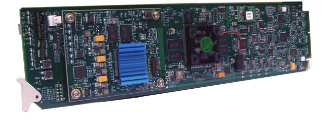
3G/HD/SD/CVBS Channel Integrator – UDX / Frame Sync with Video Optimization, Advanced Audio DSP Features, and SFP I/O Options
