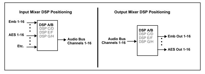
Figure 1-8 DSP Pipelines and Input/Output Mixer Positioning
