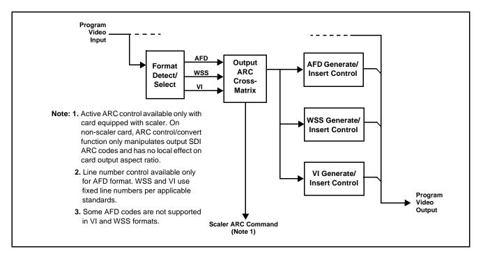
Figure 1-5 AFD ARC Processor
