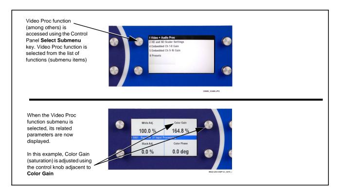
Figure 3-3 Remote Control Panel Setup of Example Video Proc Function Setup
