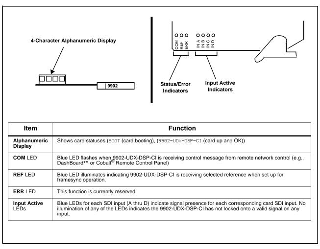
Figure 3-7 9902-UDX-DSP-CI Card Edge Status Indicators and Display
