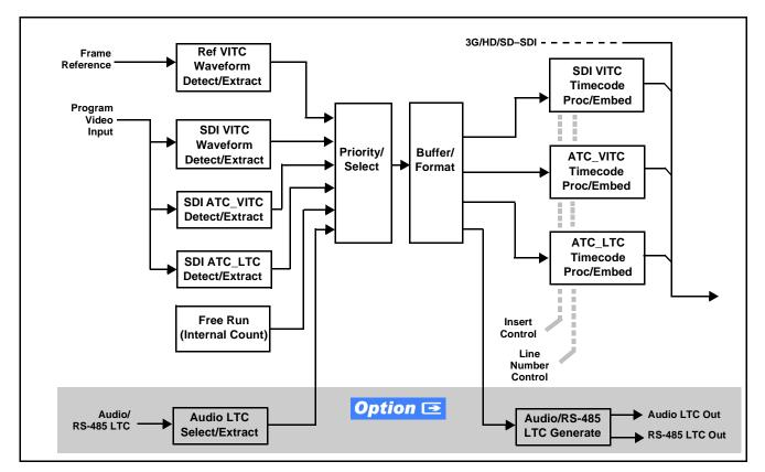
Figure 1-4 Timecode Processor
