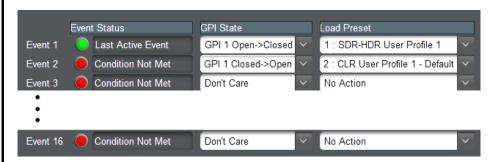
In the example above, a GPI 1 open>closed trigger will invoke selected user preset 1 (in this case, "1: SDR-HDR User Profile 1"). Also in this example, a GPI 1 closed>open trigger will be used to exit the previously invoked preset and go to a new preset (in this case, "2: CLR User Profile 1 - Default").
