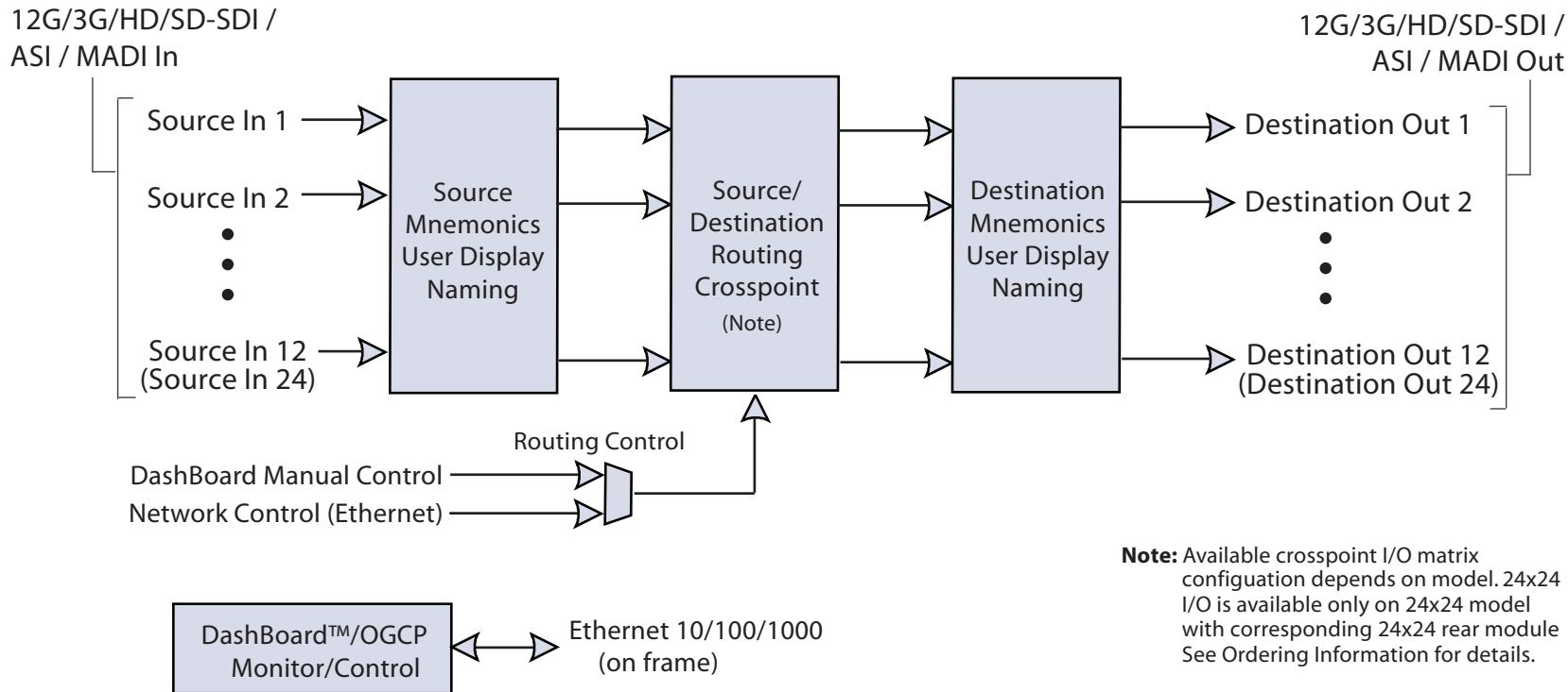
**Note:** Available crosspoint I/O matrix configuration depends on model. 24x24 I/O is available only on 24x24 model with corresponding 24x24 rear module. See Ordering Information for details.
