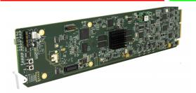
The **9950-EMDE-ANC 3G/HD/SD-SDI Ancillary Data Embedder/De-Embedder** offers full VANC/HANC ancillary data de-embedding and embedding for 3G/HD/SD-SDI streams. The easy to use user interface allows direct access to DID and SDID locations to extract or insert user data such as camera PTZ, SCTE 104, closed-captioning read/insert, GPI/GPO via ANC, or other specialized user payloads.
