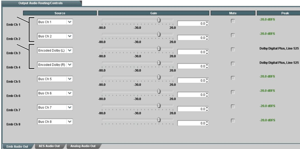
**Figure 6 Processed Embedded Audio Output Routing**
