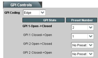
When GPI 1 closes (as set by the **GPI Controls** settings shown above), Preset 2 (“EAS insertion”) is invoked resulting in the routing changes (saved as Preset 1 and Preset 2 shown below). The Preset 2 routing changes replace the normal embedded channel routing with the ducked-mix/EAS insertion pair provided by the Input Flex Mix feature.
