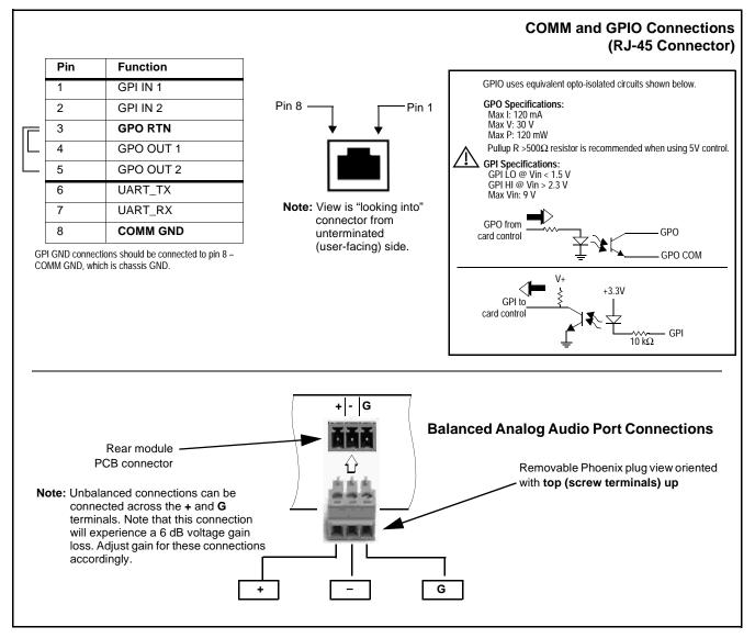
Figure 2-4 COMM, GPIO, and Analog Audio Connector Pinouts
