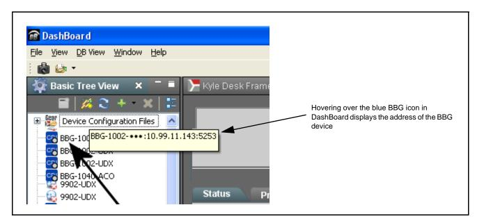
Figure 3-2 Finding BBG-1002-UDX-FS Using DashBoard
