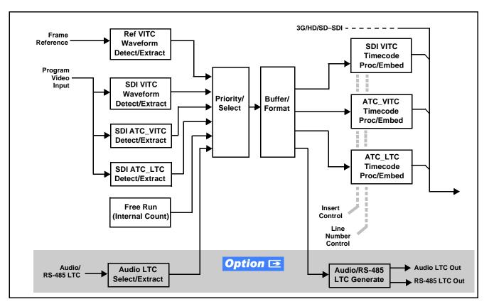
Figure 1-2 Timecode Processor
