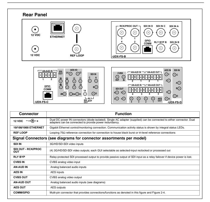
Figure 2-3 BBG-1002-UDX-FS Rear Panel Connectors
