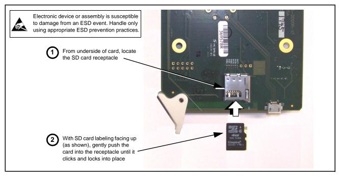
Figure 3-10 SD Card Installation
