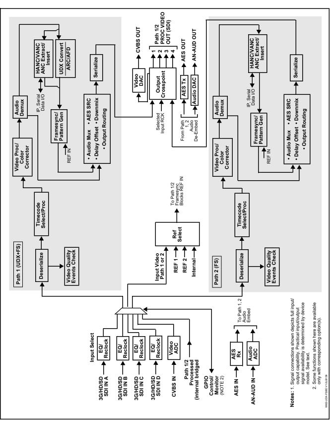
Figure 1-1 BBG-1002-UDX-FS Functional Block Diagram
