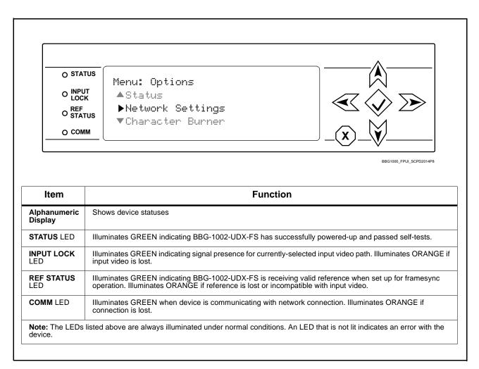
Figure 3-9 BBG-1002-UDX-FS Device Edge Status Indicators and Display
