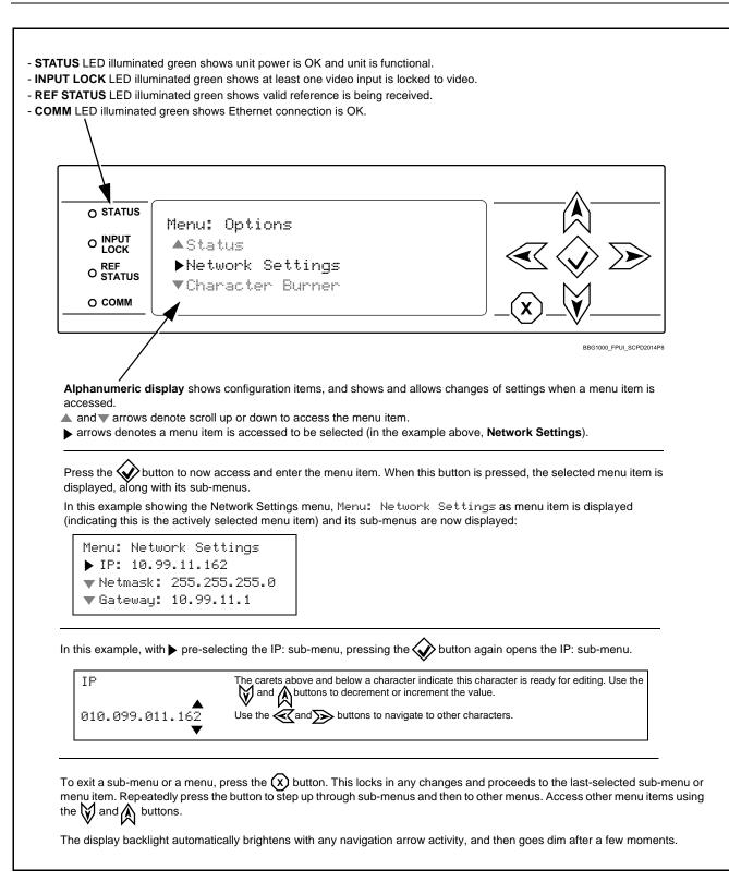
Figure 3-1 BBG-1002-UDX-FS Front Panel Display and Menu Controls
