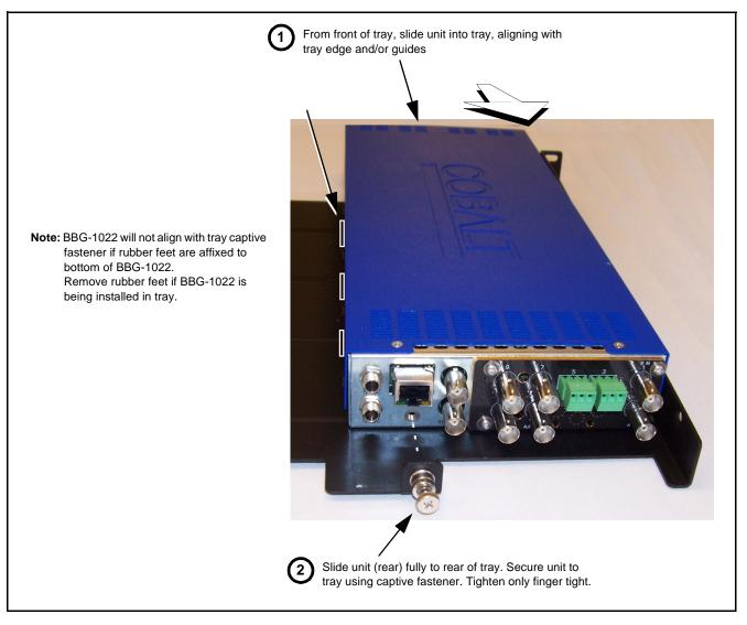
Figure 2-1 Mounting BBG-1022-2FS Using Frame Mounting Tray
