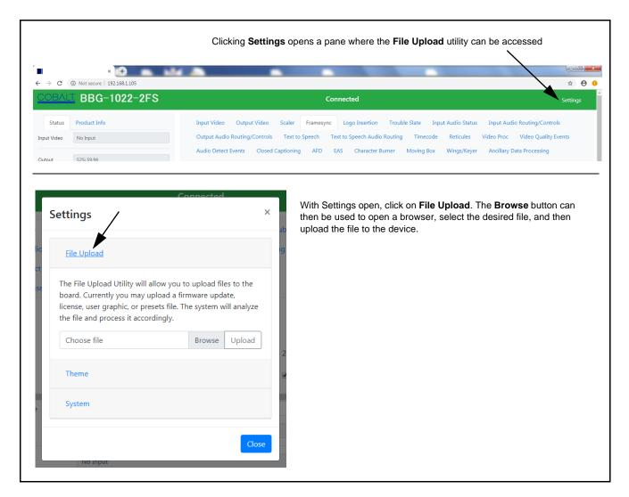
Figure 3-8 Uploads Using Web Interface/GUI
