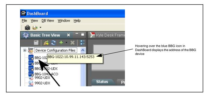
Figure 3-2 Finding BBG-1022-2FS Using DashBoard
