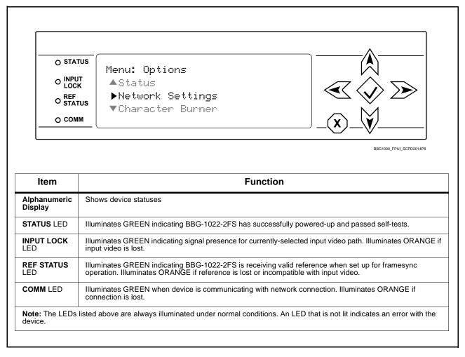
Figure 3-9 BBG-1022-2FS Device Edge Status Indicators and Display
