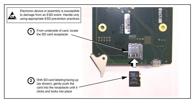
Figure 3-10 SD Card Installation
