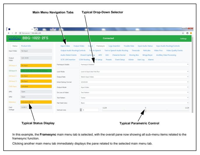
Figure 3-4 Typical Web UI Display and Controls
