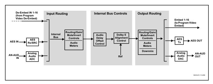
Figure 1-3 Basic Audio Processing Block Diagram
