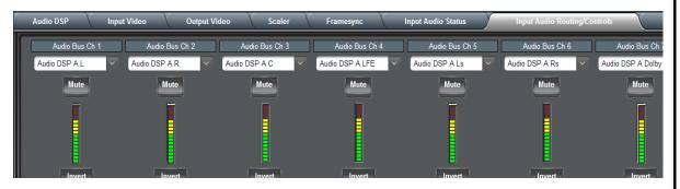
Output Mixer path positioning locates the DSP pipeline to receive Audio Bus channels (in this example, DSP E L and DSP E R receiving Audio Bus Channels 9 and 10) and then place the DSP processed output channels directly at the device audio outputs as sources for destination Embedded Output or AES Output channels via the Output Audio Routing/Controls.
