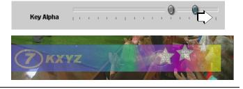
When both settings are optimized, the key/fill appears consistent in opacity and free from edge distortions or graphic bleed lines appearing in the image.
