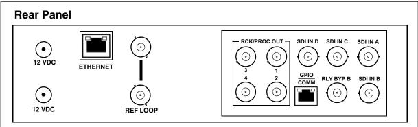
**Note:** RCK/PROC 1 thru RCK/PROC 4 are DA outputs which can be individually set as reclocked or processed outputs of the currently-selected input. RLY BYP B is a relay-protected path which carries processed SDI out under normal conditions and passive routes SDI IN B to this BNC upon loss of power.
