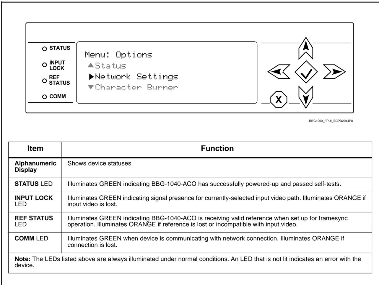
**Figure 3-9 BBG-1040-ACO Device Edge Status Indicators and Display**
