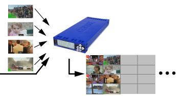
More downstream BBG-1070-QS units can be added and have its PiPs added next to those furnished from the upstream card cascade. Here, PiP insertions are arranged in columns, although almost any desired grid and arrangement scheme is possible.
