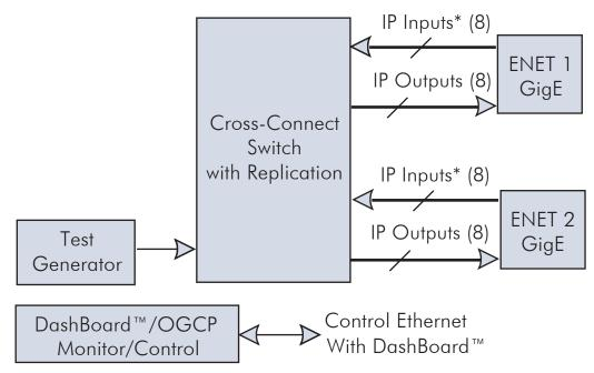
\* On model BBG-1090-RTR-8X16-MPEG-IP, number of input ports is limited to eight (total), which can be distributed across either of both GigE interfaces.
