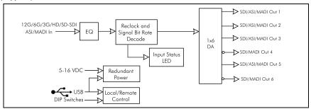
The DA-12G-1x6 can be operated in automatic standard detect mode or in a manual standard mode. Non-inverting ASI reclock is available on **OUTPUT 1** thru **3** and **5** output ports.
