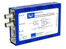
BlueBox<sup>™</sup> offers excellent performance, and excels to a new level of ease of use and installation practicality. The BlueBox<sup>™</sup> BBG-DE-AA 3G/HD/SD Analog Audio De-Embedder provides de-embedding to professional balanced audio at 0 dBFS to pro 24 dBu levels using full 24-bit conversion.
