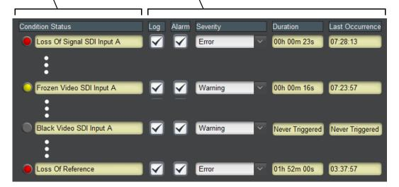
**Note:** The Log, Alarm, Severity, and Duration/Last Occurrence columns appear on the other alarm sub-tabs and function identically as described here.
