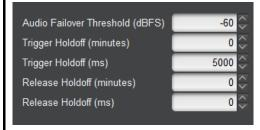
**Audio Alarm Setup** sub-tab allows setting up screening trigger threshold, engagement and disengagement holdoff for low or missing audio levels on the card's embedded audio input channels.
