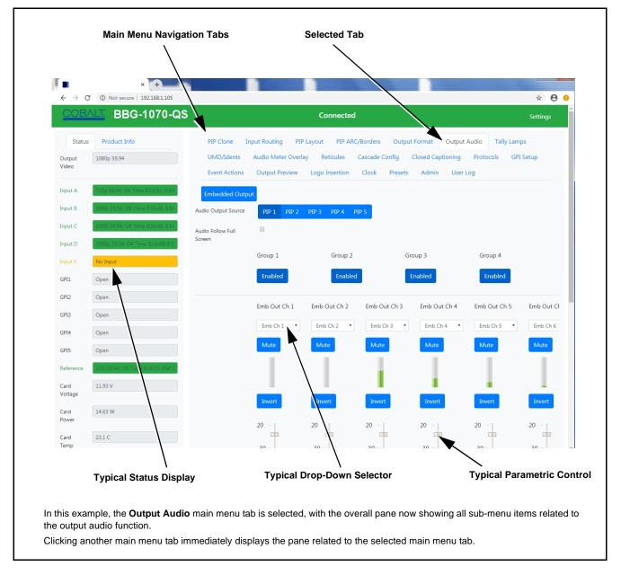
Figure 3-4 Typical Web UI Display and Controls
