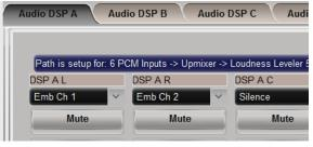
The DSP outputs are then routed to card Audio Bus Channels as desired (in this example, Audio DSP A L thru Audio DSP A Rs serving as sources for card audio bus channels Audio Bus Ch 1 thru Ch 6).
