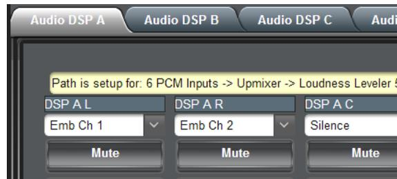
The DSP outputs are then routed to card Audio Bus Channels as desired (in this example, Audio DSP A L thru Audio DSP A Rs serving as sources for card audio bus channels Audio Bus Ch 1 thru Ch 6).
