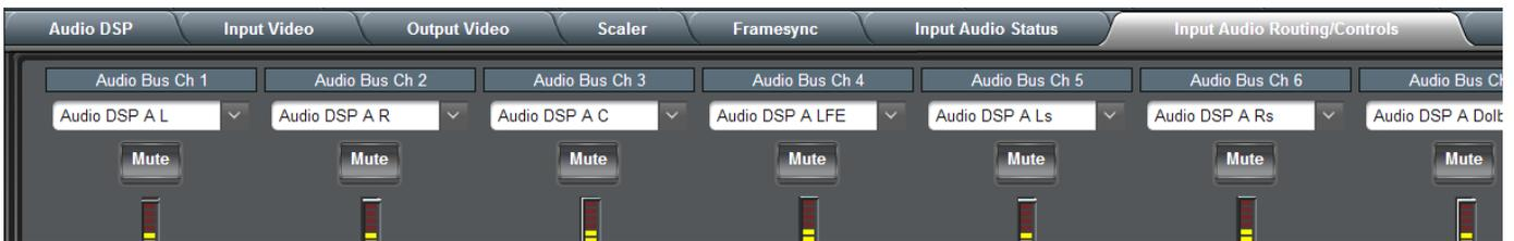
**Output Mixer** path positioning locates the DSP pipeline to receive card Audio Bus channels (in this example, DSP E L and DSP E R receiving card Audio Bus Channels 9 and 10) and then place the DSP processed output channels directly at the card audio outputs as sources for destination Embedded Output or AES Output channels via the Output Audio Routing/Controls.
