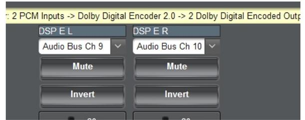
The DSP outputs are then routed to card external outputs as desired (in this example, Audio DSP E Dolby L and Dolby R serving as sources for card outputs AES Out Ch 1 and Ch 2).
