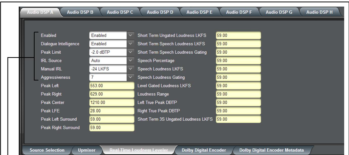
The RTLL blocks offer parametric controls for loudness leveling. Basic setup is setting RTLL to Enabled, and choosing a Manual IRL (Input Reference Level) (typically same as the desired loudness level). Other settings can typically be left at the default settings provided.
