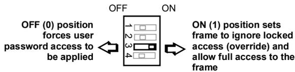
Setting DIP switch position 3 to ON or OFF allows password override as shown.
