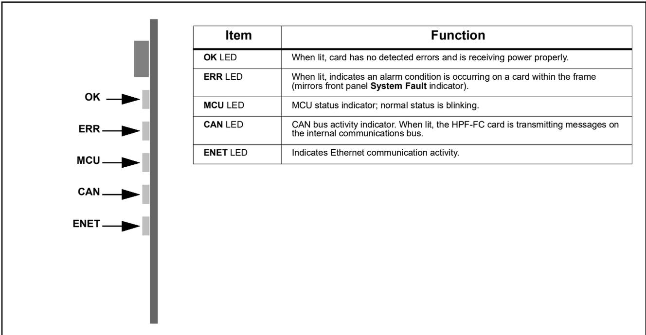
Figure 2-2 HPF-FC Network Controller Card Edge Indicators
