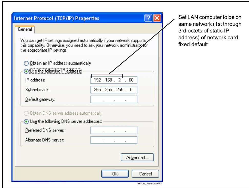
**Note:** When using a frame static IP address, if not already done it is recommended to isolate the LAN segment containing the frame, the hosting computer, and intermediate hubs or switches from other parts of the network. This prevents a potential conflict between the frame and any other node that might also have this address.
