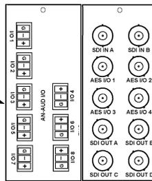
RM20-9901-B Rear Module provides connection break-out for base card functions.
