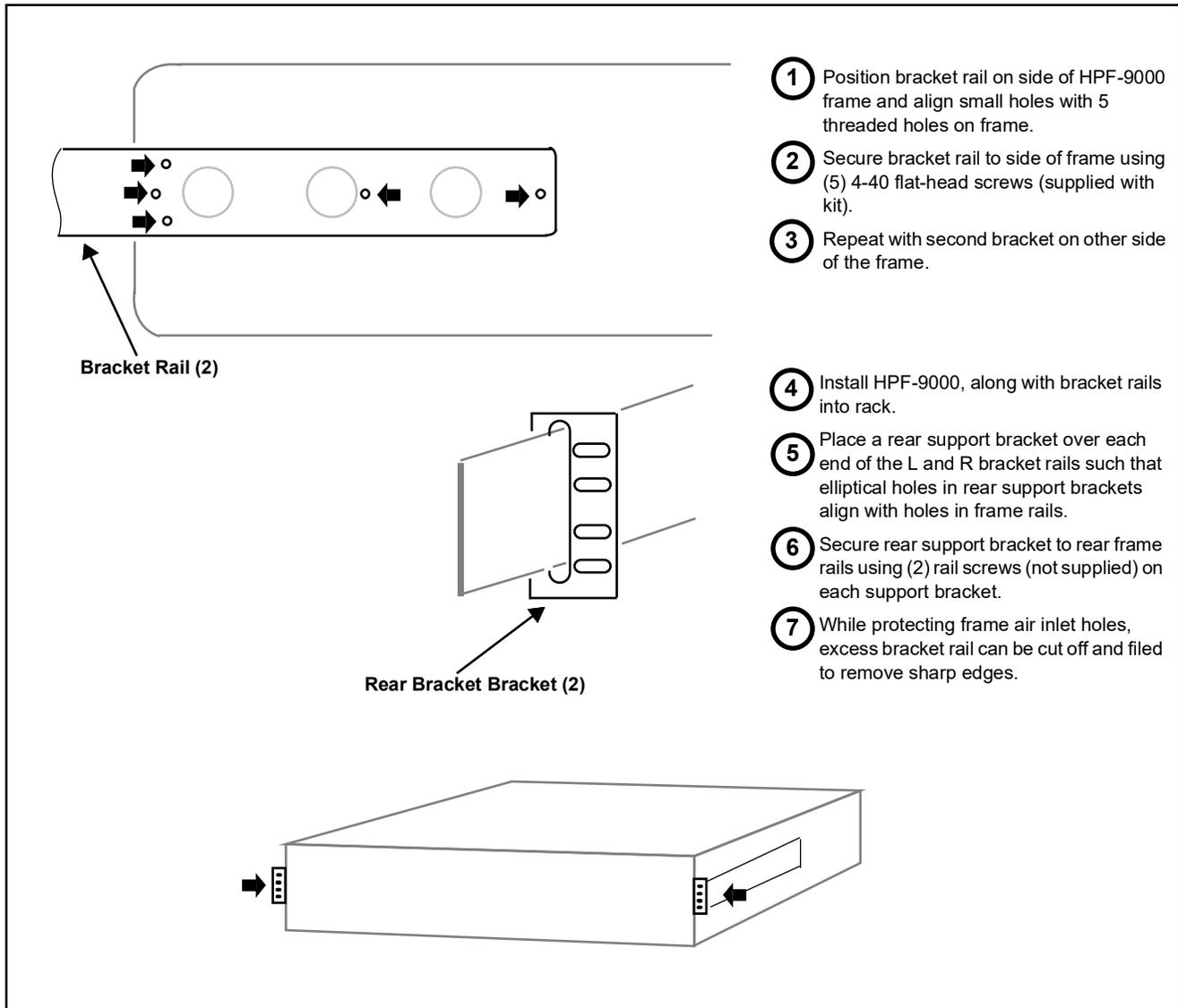
**Figure 2-4** Frame Support Bracket Kit 9000-FSB Installation
