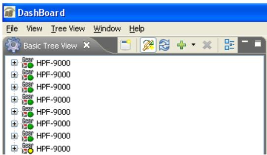
Without an orderly and documented means of connecting frames to the network, many frames may connect with no correlation to the frame's physical identity (especially if DHCP is used without adequate consideration of keeping track of connections). In this example, although the frames are connected to DashBoard™, the frame becomes "lost" from its physical identity.
