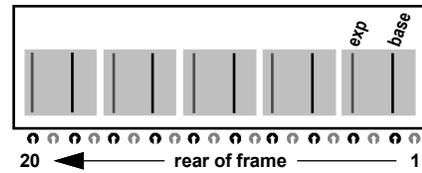
Expansion Rear Module installs directly to the **left** of base Rear Module, and interfaces with the piggyback card. In this example, an RM20-9901-XC expansion rear module breaks out analog audio connections provided by Option +ANA (analog audio option).
