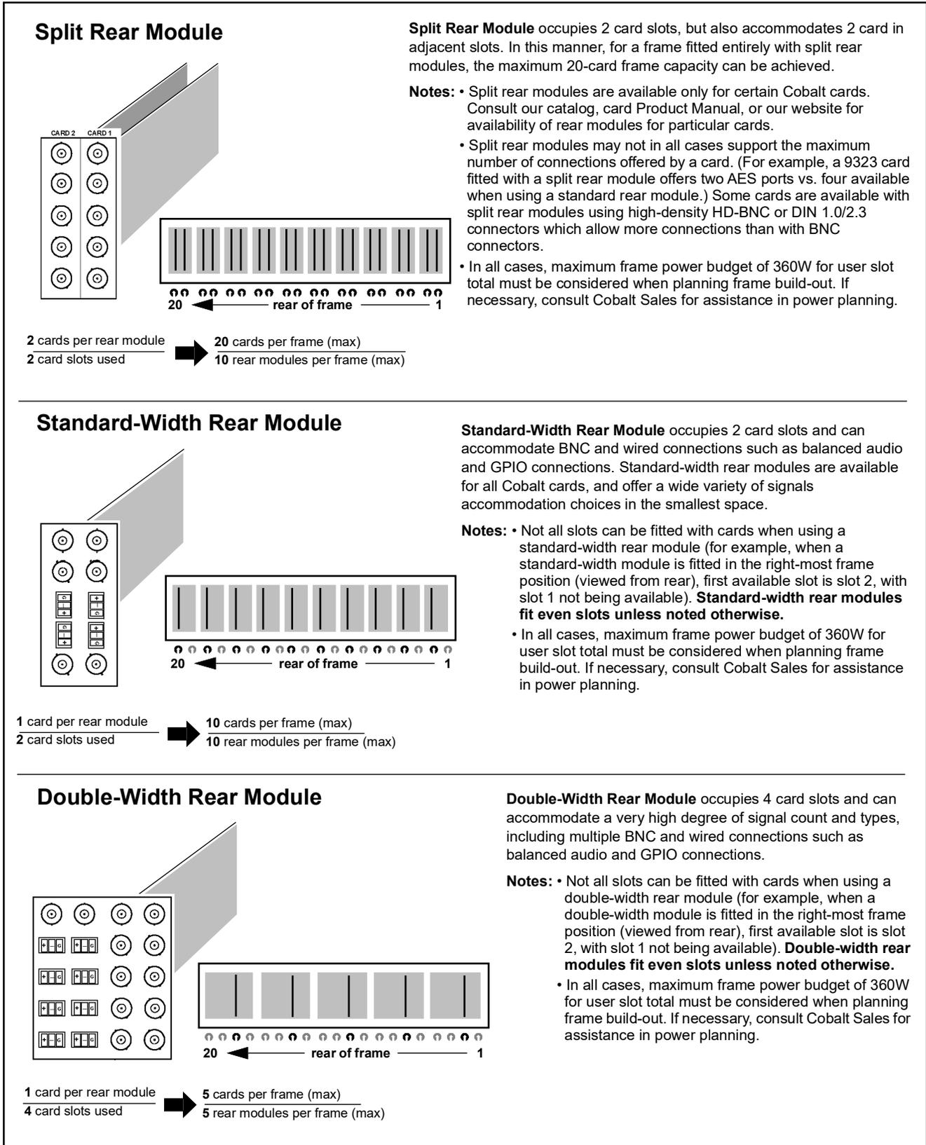
Figure 1-4 Frame Capacity for Various Rear I/O Module Types
