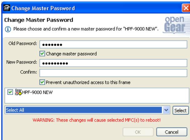
Check **Change master password** and **Prevent unauthorized access to this frame** to enable password-controlled frame access.
