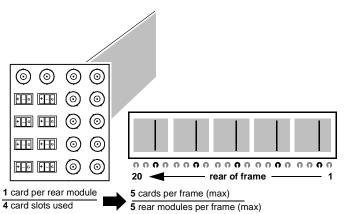
Double-Width Rear Module occupies 4 card slots and can accommodate a very high degree of signal count and types, including multiple BNC and wired connections such as balanced audio and GPIO connections.
