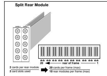
Split Rear Module occupies 2 card slots, but also accommodates 2 card in adjacent slots. In this manner, for a frame fitted entirely with split rear modules, the maximum 20-card frame capacity can be achieved.
