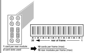
Standard-Width Rear Module occupies 2 card slots and can accommodate BNC and wired connections such as balanced audio and GPIO connections. Standard-width rear modules are available for all Cobalt cards, and offer a wide variety of signals accommodation choices in the smallest space.
