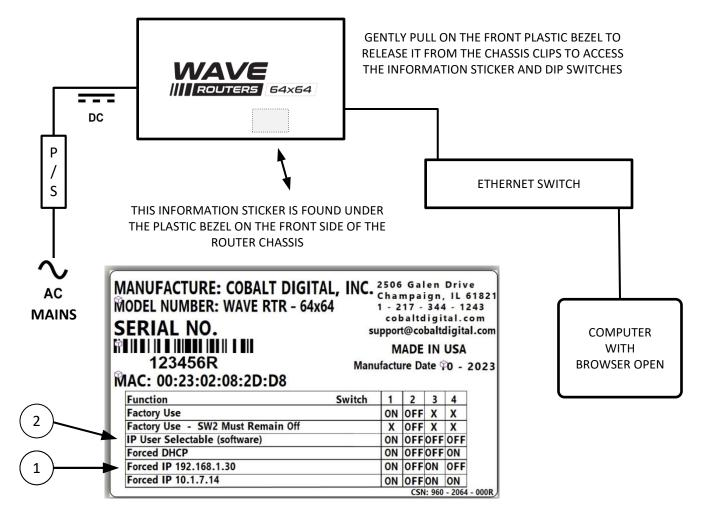
The WAVE router functions are controlled through a web GUI.
